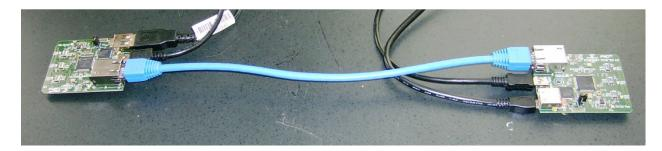
To use the SharkTap to monitor the Ethernet packets on that link, connect the SharkTap as shown in the next picture:
