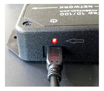
Each port jack has two LEDs. The Green LED is on when there is a valid link connection. (Note that the SharkTap has a feature called MDIX, meaning that it will automatically crossover Tx and Rx pairs, so no crossover cable is ever needed.) The Yellow LED is on if the link is 100Base-T, off if it's 10Base-T. The Green LED will blink when there are packets sent or received on that port.
