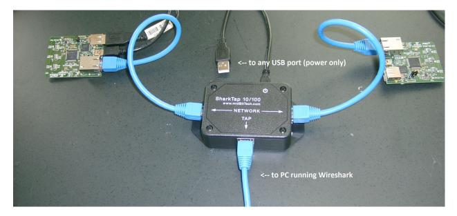
The two Ethernet devices connect to the two side ports marked 'NETWORK'. All packets on either network port will be duplicated on the TAP port. The TAP port is typically connected to a PC running the Wireshark analyzer. Finally, connect the USB cable from the back port to any USB port, or use any cell phone charger with a micro-USB connector. The red LED on the back will light red to show power is attached. (The SharkTap will not show up as a device when connected to a PC, it only draws power)
