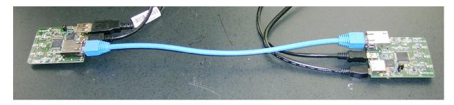
To use the SharkTap to monitor the Ethernet packets on that link, connect the SharkTap as shown in the next picture:
